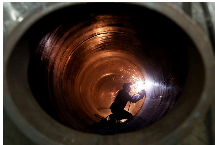
Jesse Davis works Thursday on cleaning the inside of a large tank being produced at Universal Tank & Fabrication in Dubuque. The company focuses exclusively on customized work.
